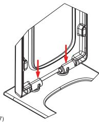
Keeping seat and cover in the icon position, insert the holes of seat and cover into the hinge.
