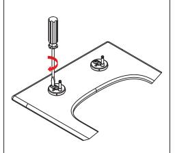
(5) Fully tighten the screws .
